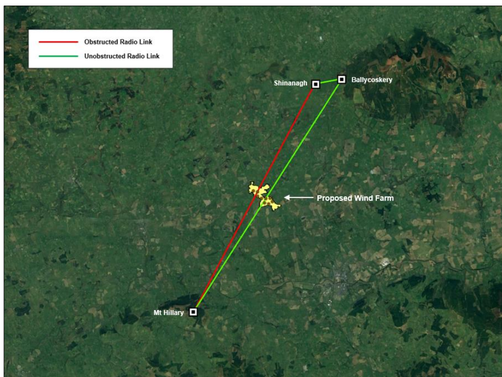
Figure 16. Relay radio link via existing Telecoms Mast – Tullacondra Wind Farm Example
